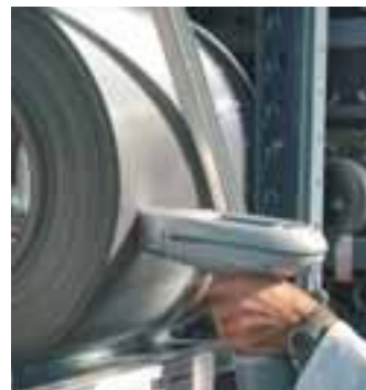
Instrument for electronic detection of the chemical composition of the raw material
